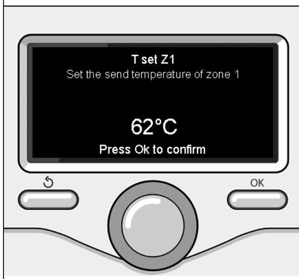
Change heating hot water temperature
